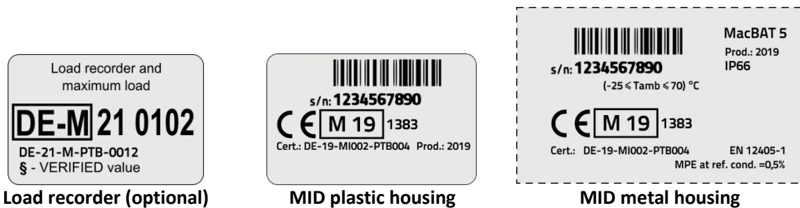
Figure 10. Nameplates placed on front door of the device (examples)
